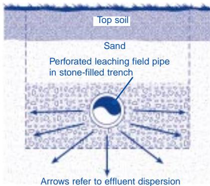
flows out of the tank and into a series of underground trenches filled with gravel. The effluent trickles through the gravel into the soil where the organic matter decomposes.
