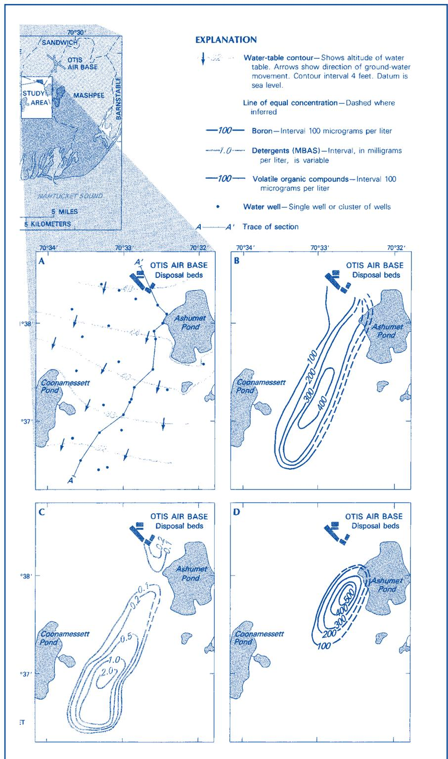
Sewage plume in ground water downgradient from Otis Air Force Base in 1983. **A** shows the water-table contours and the location of sampling wells. **B** shows the distribution of boron, in micrograms per liter. **C** shows the distribution of detergents, in milligrams per liter. **D** shows the distribution of volatile organic compounds, in micrograms per liter (Hess, 1986).
