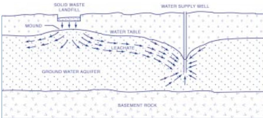
How leachate from a solid waste disposal site contaminates a well. From the *Environmental Impact of Ground Water Use on Cape Cod*. (Strahler, 1972).
